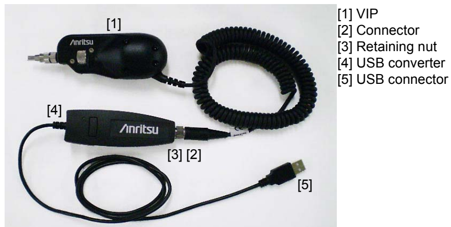
Figure 9.2-3 VIP Connected to USB Converter
