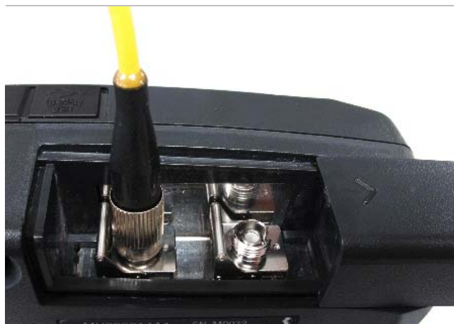
Figure 2.6-1 Connecting Fiber to Measurement Port
